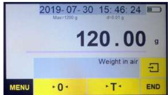
6. To check its weight in the air, click . Immerse your sample on the structure in the liquid beaker, the display will show
